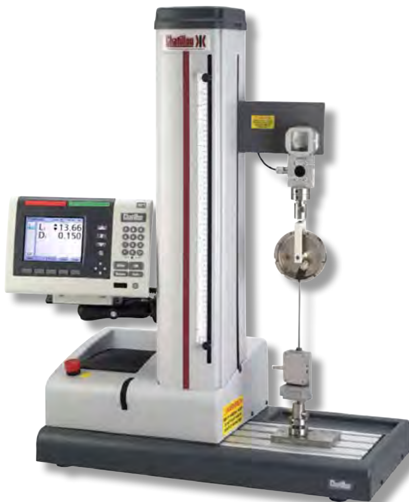
Shown: Medium capacity TCD225 Series with optional testing fixture for wire terminal testing.
