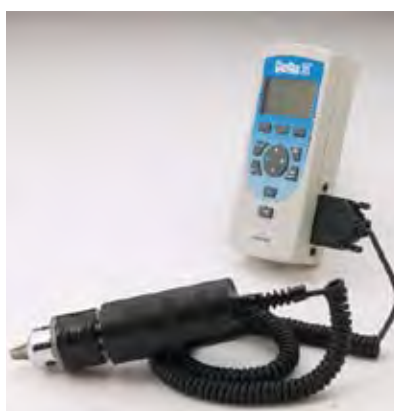
Shown: STS sensor attached to the Chatillon DFS-R-ND gauge for torque measurement.
