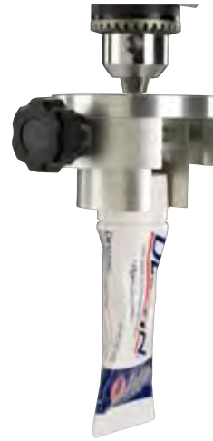
Shown: STS sensor attached to the B200308 torque fixture for measuring cap torque strength.
