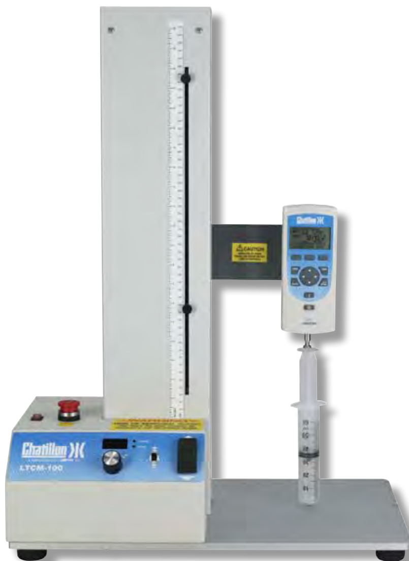
Shown: LTCM100 Series with optional DFS Series force gauge.
