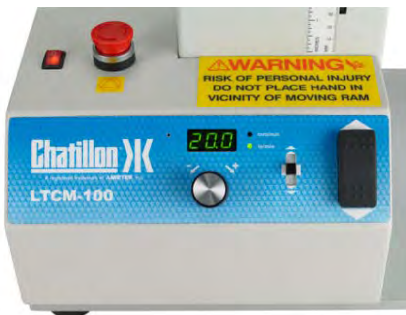
Shown: Control panel is designed to promote ease-of-use. All controls are located on the control panel and away from the work area, making the LTCM100 Series ideal for busy production environments.
